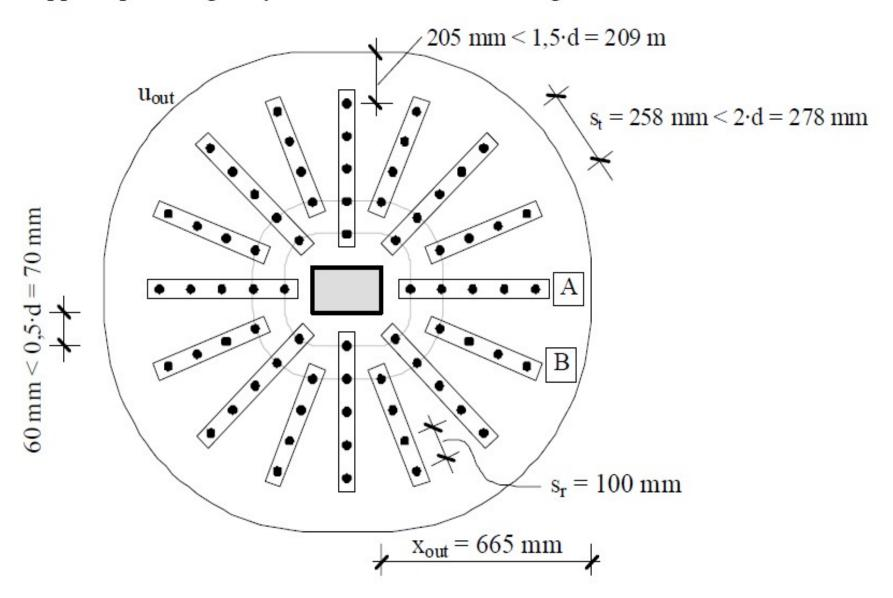
Prefabricated shear reinforcement consists of 2 or 3 studs welded to a steel rod. These could be combined:
