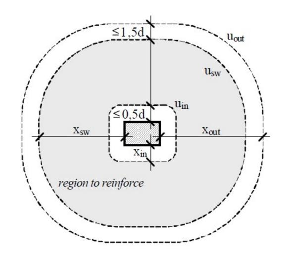
• Distance of the most extreme  $\mathbf{u}_{out}$  punching perimeter from the column Length of the punching perimeter being x distance from the column:
