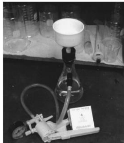
Total suspended solids filtering apparatus
