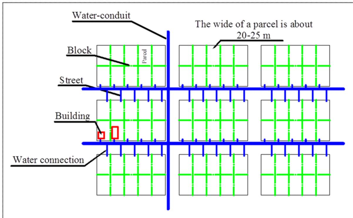
Figure 1.: Determination of the number of the connection pipe
