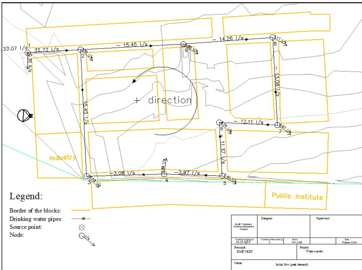
Figure 3. The initial water flow and direction
